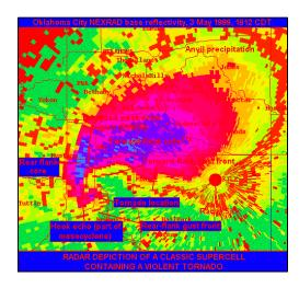
Fig. 3. RADAR imaging allows meteorologists to pinpoint the probable locations of tornados before they touch down in many cases.
